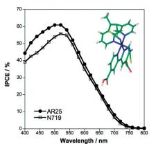
We describe a new ruthenium heteroleptic complex that shows enhanced photocurrent when used as sensitizer in dye-sensitised solar cells. The complex shows an IPCE at the maximum absorbance wavelength exceeding the performance of a commonly used ruthenium homoleptic complex under the same conditions.
